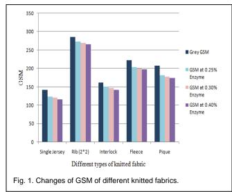
A great difference observed in between the grey gsm and the gsm after enzyme treatment. Grey gsm of the fabric tends to decrease in enzyme treatment. For example grey gsm of single jersey knitted fabric was 141 and after bio-polishing with enzyme of different concentration (0.25%, 0.30% and 0.40%) the gsm of the same fabric found were 123, 120 and 116 respectively. This phenomenon has also been observed for all the other 4 kinds of fabrics (rib (2\*2), interlock, fleece and pique).
