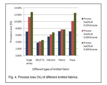
Single jersey knitted fabric showed maximum process loss (12.76%) at 0.40% enzyme during bio-polishing. Among all of the different knitted fabrics rib (2\*2) showed lowest process loss (4.54%) at 0.40% enzyme.
