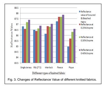
The increase in the concentration of enzyme during biopolishing lead to the increase in reflectance value. For all kinds of knitted fabrics reflectance value increased along with the increase in enzyme concentration (%). For example reflectance value 86.59, 87.19 and 87.40 were observed for single jersery fabric with 0.25%, 0.30% and 0.40% enzyme repectively.
